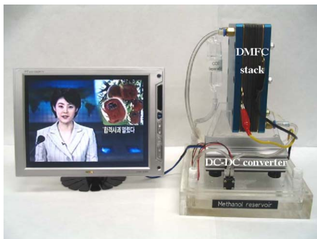
Fig. 11. Photograph of an LCD TV monitor turned on by the six-cell DMFC stack with a DC–DC converter.
